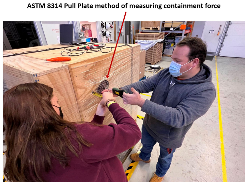
Figure 4 Measurement of the containment force on the side of the simulated unit load.
