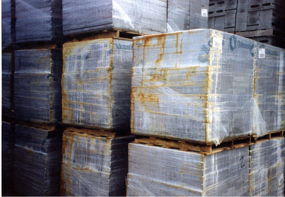
Figure 2 Discolorations on pavers and blocks cause by pallets during outside storage
