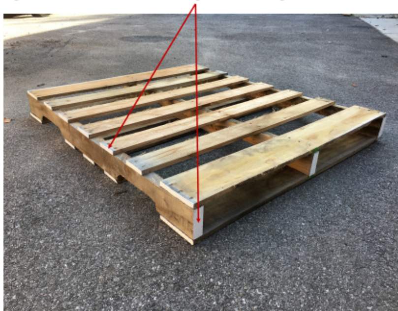
Figure 5 Pallet with end coating on the stringers and deck boards
