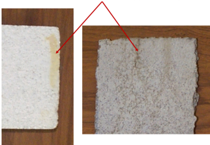
Figure 2 Discolorations on pavers and blocks cause by pallets during outside storage
