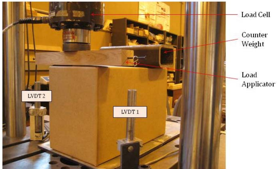
Figure 8. A photograph of the test for measuring the compression stiffness of the corrugated container.
