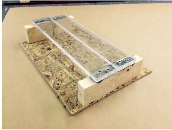
Figure 2. High stiffness deckboard segments mounted to oriented strand board base with no span (0 mm) between deckboards.
