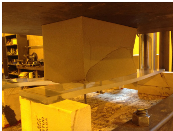
Figure 6. Front angle photograph of a box on low stiffness deckboard. Corner crush opposed to the buckling along the width sidewall.
