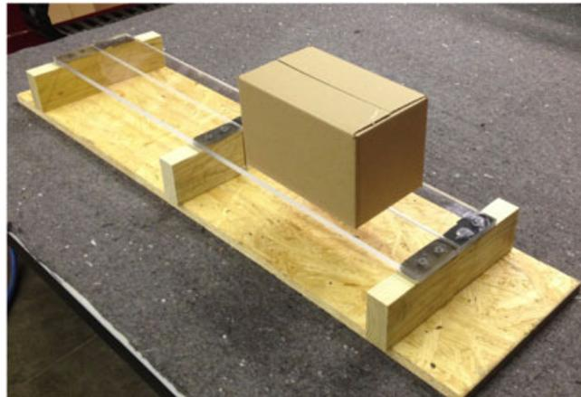
Figure 3. A photograph of full-length medium stiffness deckboards mounted to oriented strand board base with no span (0 mm) between deckboards. Box positioned at location 1 (centred between the stringers).
