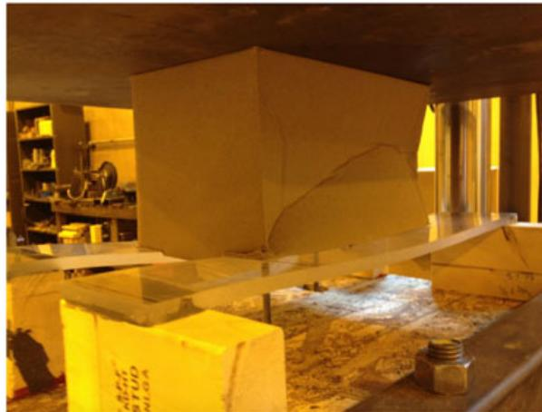
Figure 6. Front angle photograph of a box on low stiffness deckboard. Corner crush opposed to the buckling along the width sidewall.
